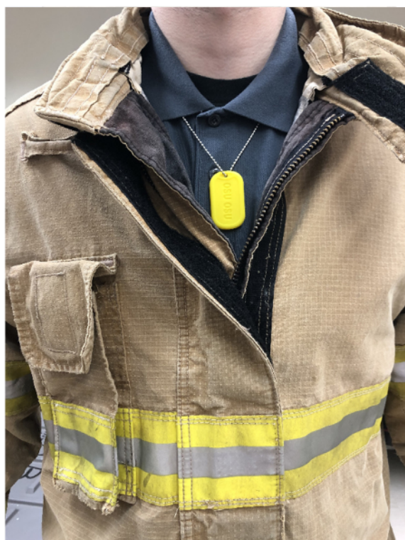
Fig. 1. Silicone dog tags (shown in yellow) were worn around the neck underneath firefighting personal protective equipment. (For interpretation of the references to colour in this figure legend, the reader is referred to the web version of this article.)
